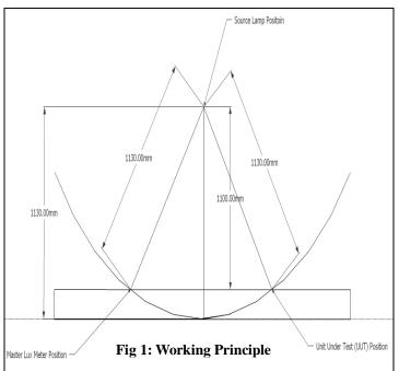
Instead the proposed system is designed such that it replicates a section of the integrating sphere. The source is kept at the centre of an imaginary sphere. Solid angle of imaginary sphere is limited by using non-reflecting bellows. The master and UUT are kept on radial surface points of the imaginary sphere. Hence Lux at the detector plane of master and UUT is equal.
